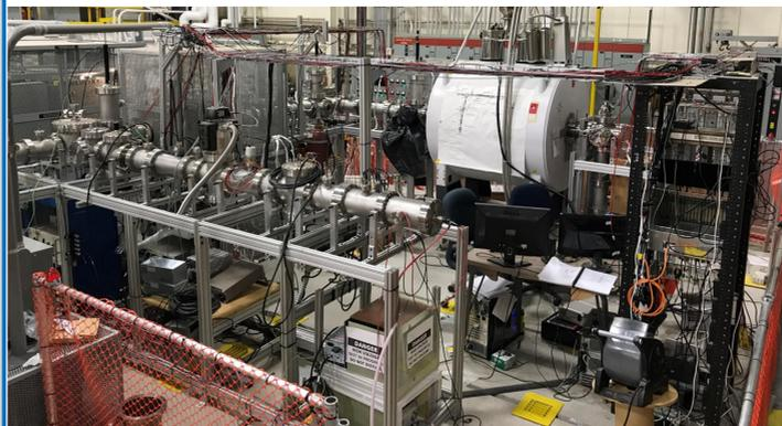
The beamline is a complex set of deflectors, lenses, and steerers in order to control the path the ion takes while traveling to the Penning trap.
