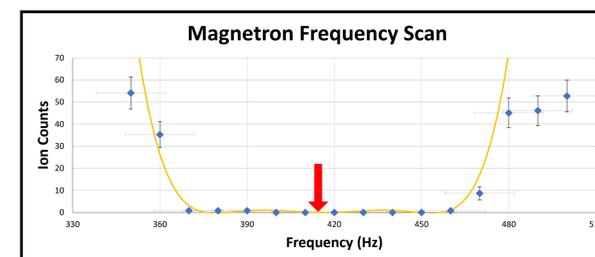
We observe  $\omega_+$  by pinpointing the trough of the time-of-flight vs frequency spectra. At resonance, the ions gain more radial energy which is then transformed to axial energy and therefore leads to a shorter time-of-flight.
