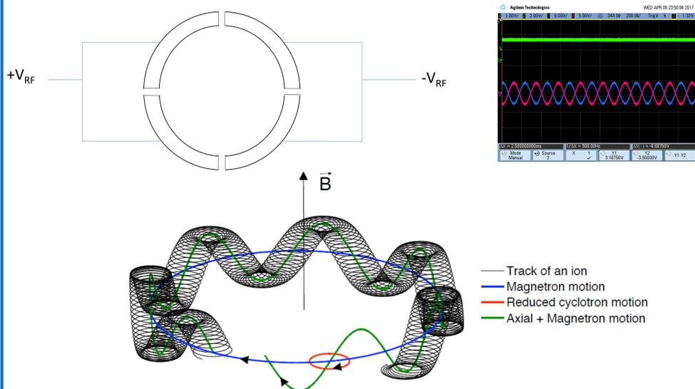
The ions are excited by alternating radiofrequency voltages on the segmented center ring electrode. At resonance, these equal-magnitude, but 180° out-of-phase, sinusoidal voltages cause the ions to rotate in different motions. Once the ions become excited, they are shot through the end of the trap to a detector.
