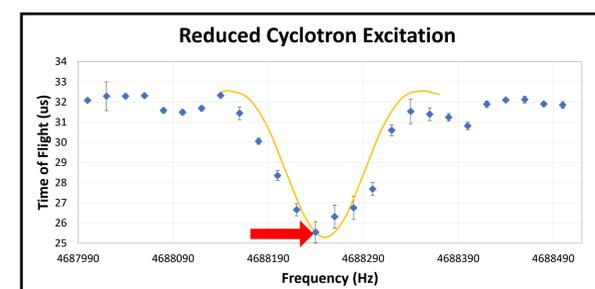
Summing the frequencies from  $\omega_-$  and  $\omega_+$  will result in a close approximation of where we should observe the cyclotron motion because  $\omega_c$  is coupled with the previous two motions. Again, the pure cyclotron motion at the resonance results in a shorter time-of-flight. The mass for the sodium ion can then be determined.
